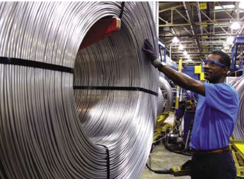
An employee moves aluminum rod, which is drawn into wire at Southwire's Utility Products Plant in Carrollton, Ga.
